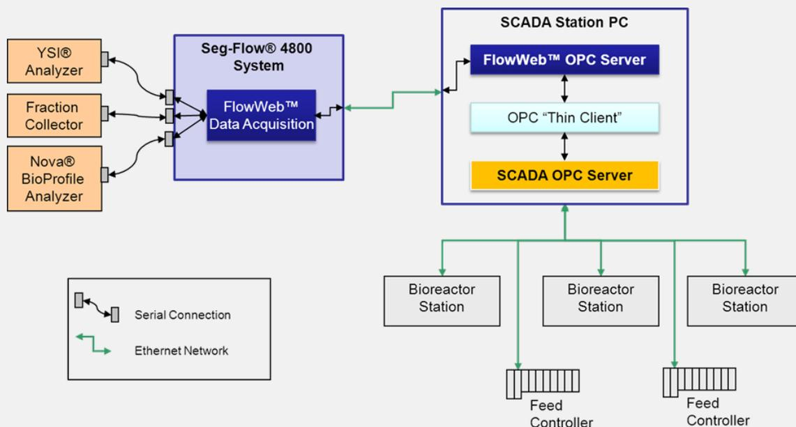
**Figure 1.** Architecture for the Seg-Flow 4800 process trigger sampling function. The process event or “trigger” is user-defined and is programmed in the bioreactor’s OPC-enabled SCADA or bioprocess management system, which remotely controls the Seg-Flow system.
