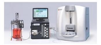
Figure 1. The Vi-CELL XR/Seg-Flow 4800 automated online cell analysis system.
