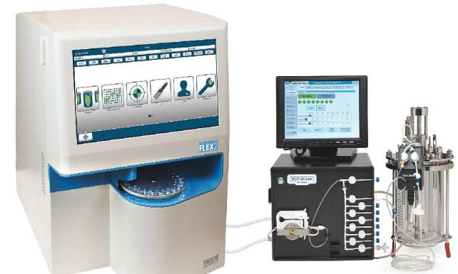
The Seg-Flow® 4800, Flownamics' automated system for online sampling and feed control, can draw samples from one to eight vessels and deliver each vessel sample to as many as four analyzers and/or fraction collectors. In this image, the Seg-Flow instrument is connected to a 2-L bioreactor and the BioProfile FLEX2, Nova Biomedical's cell culture chemistry analyzer.
