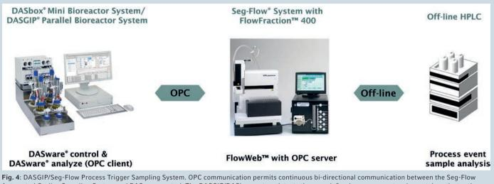
Automated On-line Sampling System and DASware control. The DASGIP/DASbox system detects the user-defined process event and remotely activates the Seg-Flow System to perform the process trigger sampling function.
