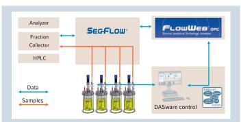
**Fig. 3**: Architecture for the Seg-Flow 4800 process trigger sampling function. The process event or "trigger" is user-defined and is programmed in the bioreactor's OPC-enabled SCADA or bioprocess management system, which remotely controls the Seg-Flow system.
